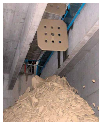
After Solid cakes of mineral after water removal.
