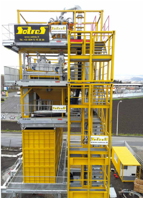
Superstructure version « Le Grand Paris » Desilter D550-550 (550 m 3 /h on the primary 550 m 3 /h on the secondary)
